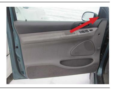
**STEP 9:** Attach the screws that hold the door trim panel onto the door.
