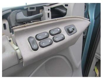
**STEP 3:** Remove the screw that holds the interior door panel onto the door.
