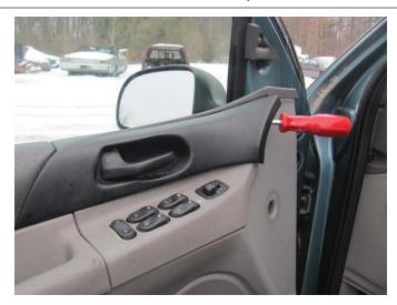
**STEP 2b:** Using a trim removal tool, remove the master switch bezel assembly.
