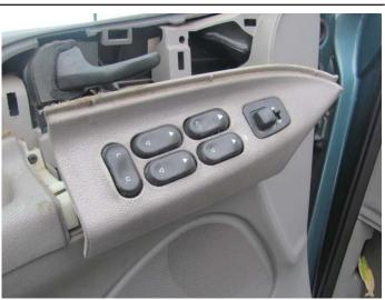
**STEP 11:** Install the door handle bezel assembly.
