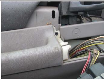
**STEP 10:** Connect the power master switch assembly and install into the door trim panel.
