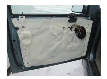
**STEP 5a:** Remove the water shield from the door.
