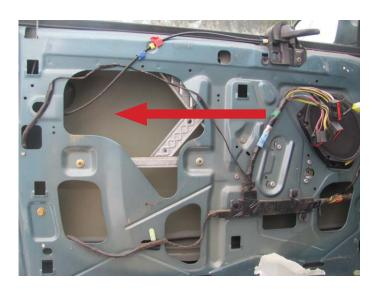
**STEP 2:** Bolt the window regulator assembly into the door.
